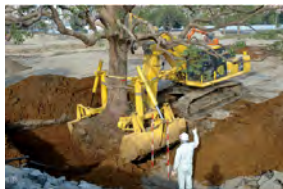
Transplanting work using a TPM machine
