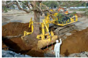
Transplanting work using a TPM machine
