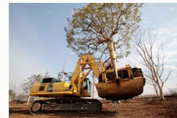
Transplanting work using a TPM machine
