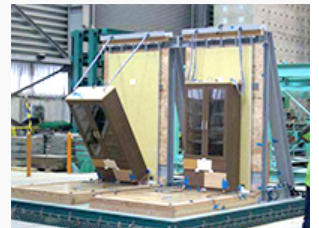
Testing in a vibration simulator
