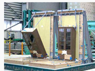
Testing in a vibration simulator Cooperation: Tokyu Construction Co., Ltd. Engineering Research Laboratory
