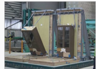
Testing in a vibration simulator Cooperation: Tokyu Construction Co., Ltd. Engineering Research Laboratory
