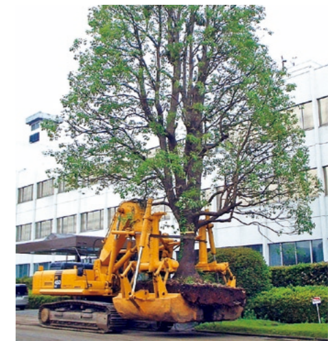
Technology for transplanting large diameter trees, "TPM method"
