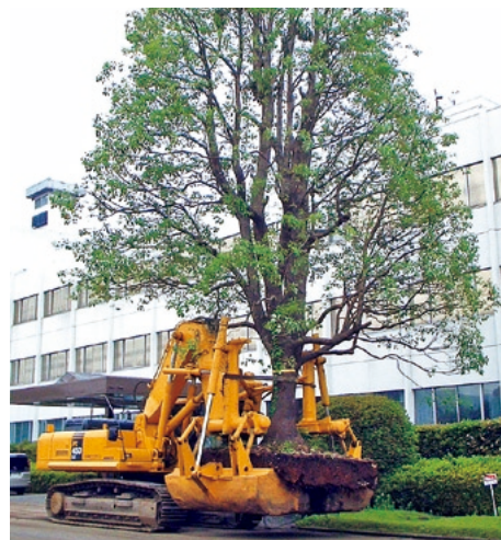
Technology for transplanting large diameter trees, “TPM method”
